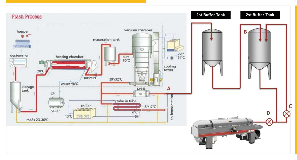
A- feeding the first buffer tank with the thermo-treated product, always mixed with internal blades.
